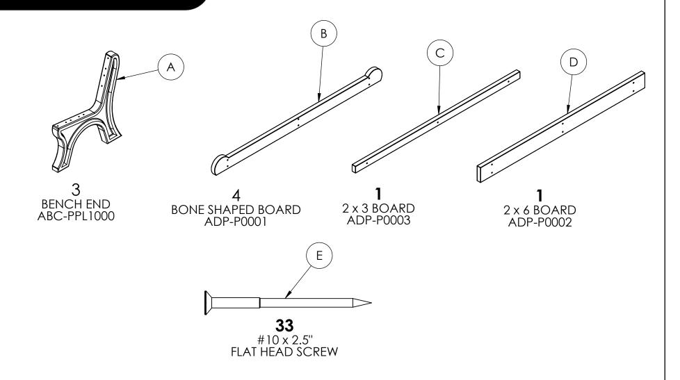
REQUIRED TOOLS (NOT INCLUDED) - POWER DRILL NOTE: IT IS IMPORTANT TO KEEP ALL SCREWS LOOSE DURING ASSEMBLY UNTIL ENTIRE BENCH IS ASSEMBLED
