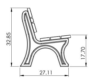
CONSTRUCTION MATERIALS: Recycled Plastic HARDWARE: Stainless Steel
