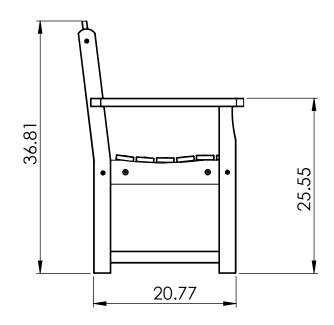
CONSTRUCTION MATERIALS: Recycled Plastic HARDWARE: Stainless Steel
