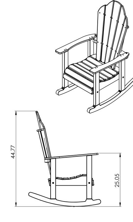
CONSTRUCTION MATERIALS: Recycled Plastic HARDWARE: Stainless Steel
