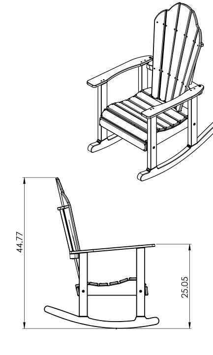
CONSTRUCTION MATERIALS: Recycled Plastic HARDWARE: Stainless Steel
