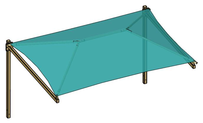
These drawings are for reference only and should not be used as construction details. Materials, fasteners, and foundations are subject to change if professionally sealed engineering drawings are required. Designed for 93 MPH Basic Wind Speed.
