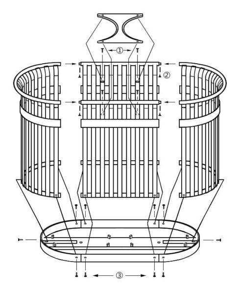
**Step 1:** On a firm, flat surface position the two flat receptacle panels across from each other with the two receptacle basket half circles at each end of the flat panels to form a complete basket. Line up the pre-drilled holes at the top (2) of the receptacle and insert the screws. Hand-tighten the screws.
