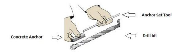
4. Before starting to drill the hole, it is important that eye and ear protection are used. Make sure the hammer drill is in the hammer mode and start drilling your hole. Continue drilling until the tape on the bit or the drill gauge meets the base material- this means that the required depth has been reached.
