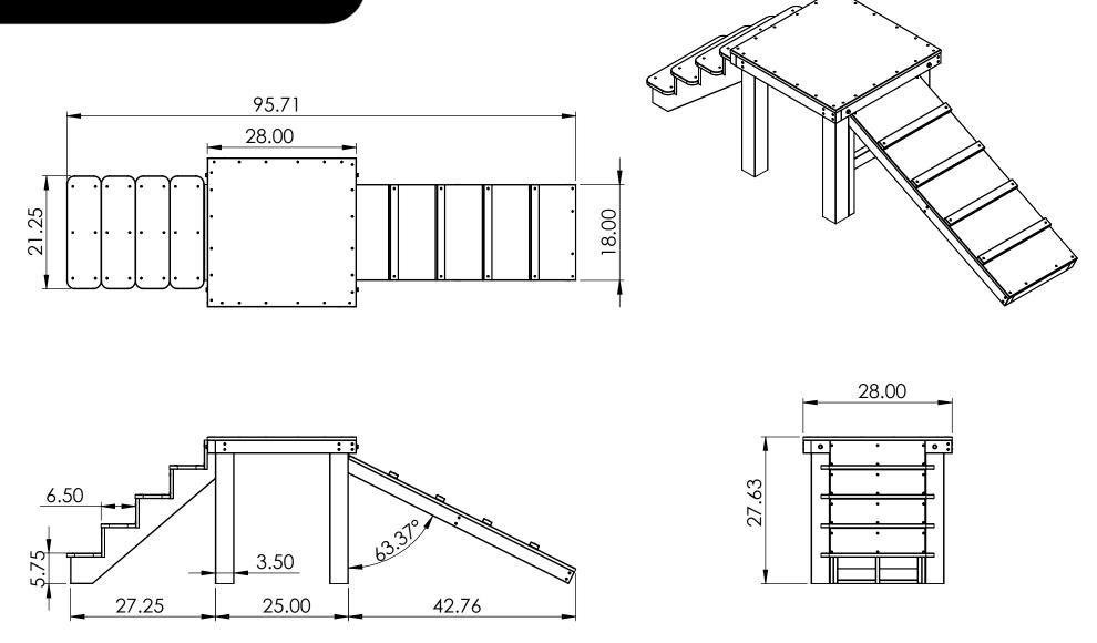
CONSTRUCTION MATERIALS: Recycled Plastic HARDWARE: Stainless Steel
