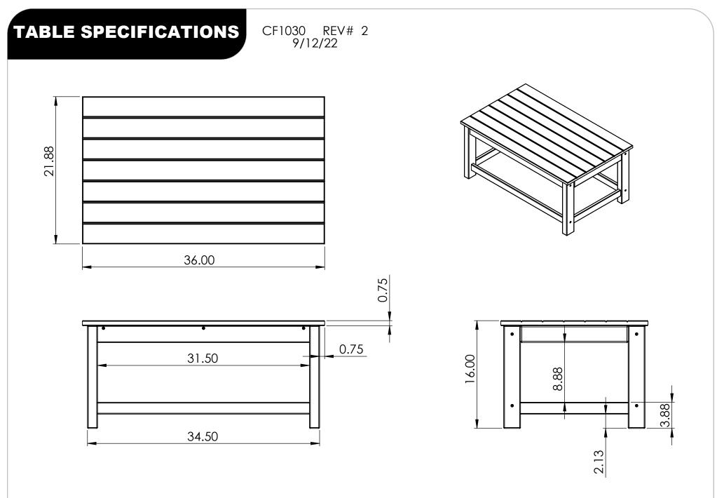
CONSTRUCTION MATERIALS: Recycled Plastic HARDWARE: Stainless Steel
