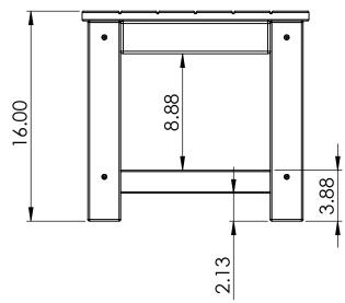
CONSTRUCTION MATERIALS: Recycled Plastic HARDWARE: Stainless Steel
