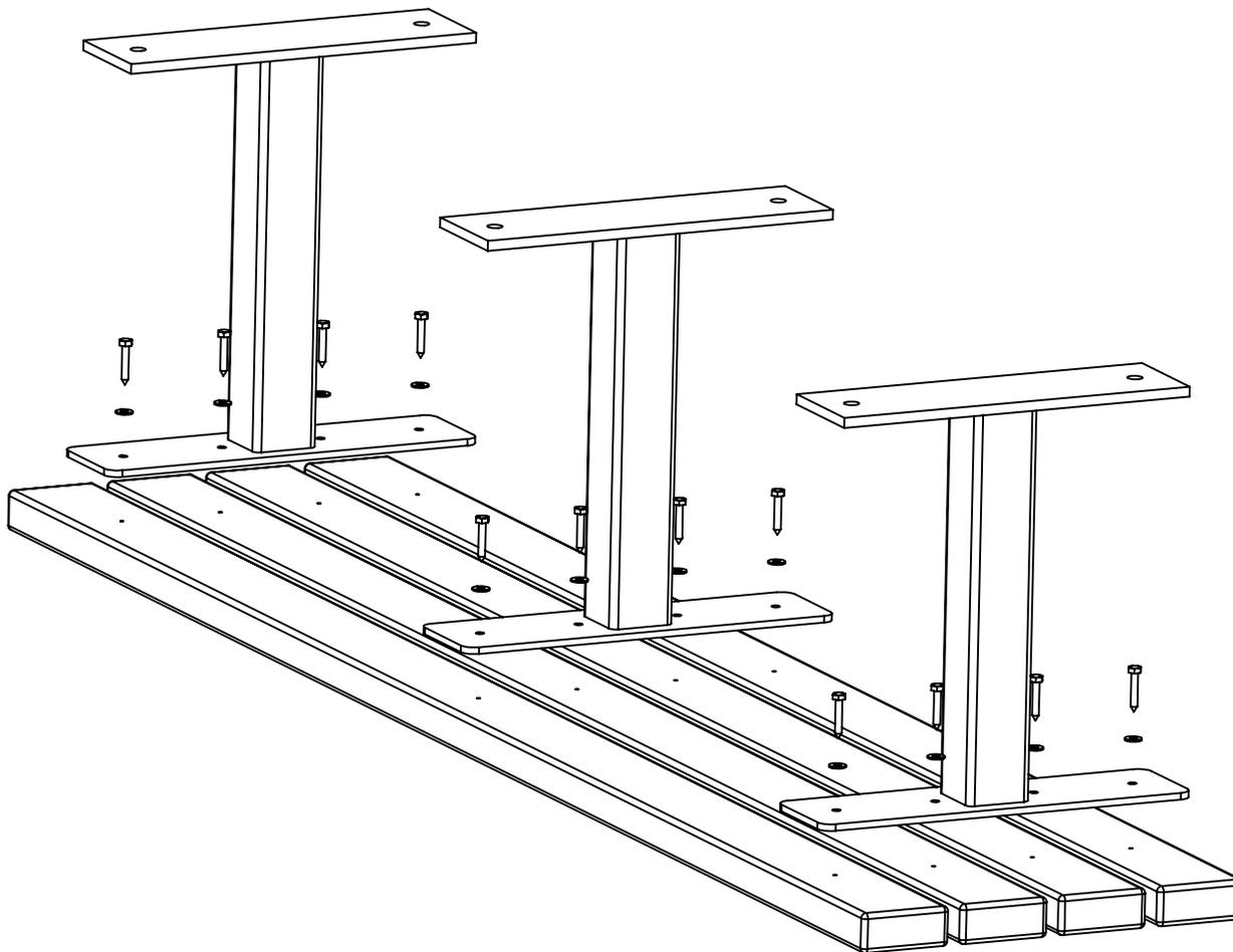
**NOTE:** Make sure BOTH ends of the bench are square before fully tightening everything down. If possible, secure one of the short ends of the bench against a wall or other flat surface.
