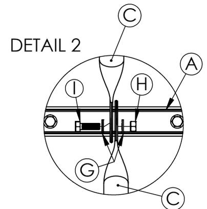
Angle support brace connection to center channel
