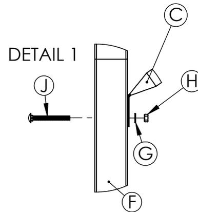
Angle support brace connection to plastic end support
