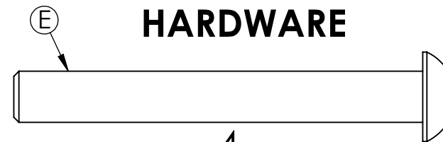
4 3/8" x 3" Button Head Cap Screws SCBH037C300188
