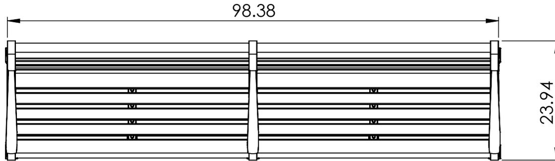
Tear drop board 3.75" x 1.34" 2.88" of flat surface on board
